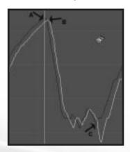
to optimising your driving to the maximum. You can, for example, follow a similar procedure to the above for the steering lock angle. If the angle is too large, the front wheels will respond less well and the car will understeer, which has a considerable effect on speed in corners.
